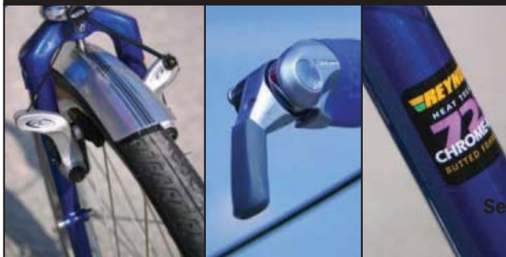
Touring classics: cantilever brakes offer a good mix of power and modulation; Bar end shifters are still de rigueur on drop bar tourers – and can easily be switched to friction shifting; Reynolds steel has been the material of choice for generations
