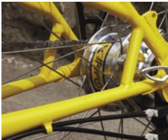
Rohloff hub plus 48T chainring and 16T sprocket gives 22-114in gears
