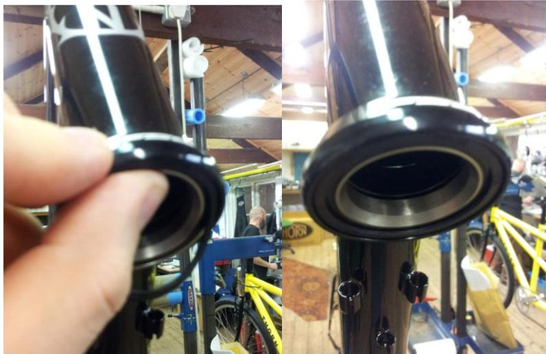
With the upper headset cup make sure the cup is clean and free from any sticky tape, dust or card shavings
