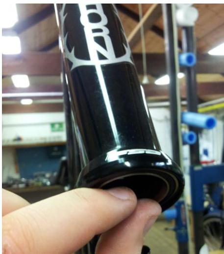
Then tuck the black rubber/plastic shield into the groove in the lower cup, this will hold the bearing in
